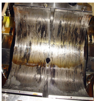
Bearing metal worn out, steel-steel contact
