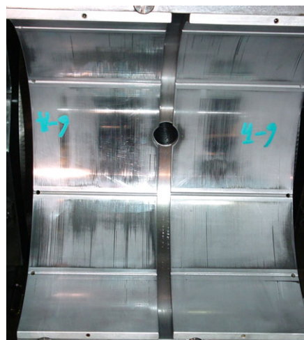
Fully intact overlayer. Acceptable!
