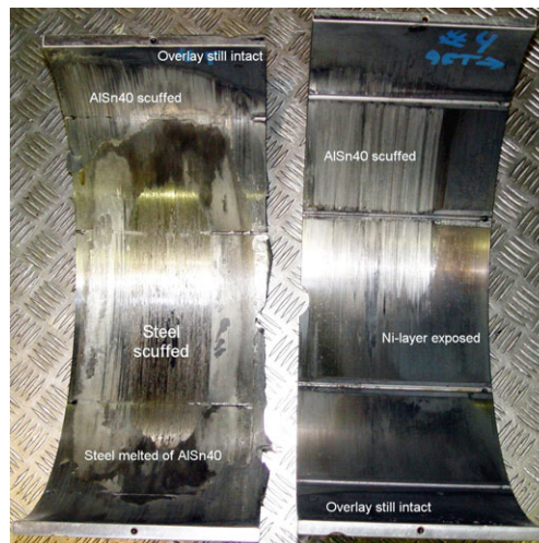
Overlay completely corroded away, partly scuffing between Ni-layer and pin, partly steel-to-steel contact. Not acceptable.
